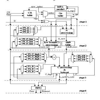
Fig. 6. Pipeline architecture of the MQ-Coder.
