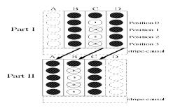
Fig. 3. The proposed coding context-window register
